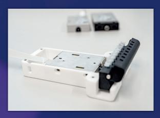
The holder is used to precisely position and analyze PCR tubes in front of the detector.
