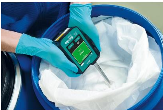
A handheld Raman-Spectrometer of the manufacturer Metrohm is used to perform a quality check of incoming goods [45]
